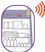
The SPY RF recorder measures and records the temperature data and wirelessly transmits to the Sirius Box receiver.
